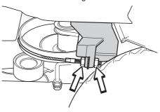
5 Unscrew the belt shields and the side protectors. The protectors are fitted on both sides of the machine.
