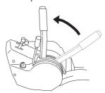
2 Pull back the throttle and turn the ignition key to the "STOP" position.
