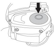
Check the air duct, located on the inside of the engine cover, ensure it is clean and does not rub against the cooling air intake
