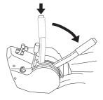
The lever can also be used to temporarily regulate the cutting height, e.g. for a small mound in the lawn.
