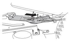
3 Loosen the parallelism stay's nuts, the inner nut has a lefthand thread.
