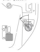
When the Rider is at a standstill, press down the parking brake and push in the locking button.
