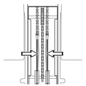
4 If necessary, the wires can be adjusted by tightening the adjuster nuts on each side of the steering collar.
