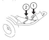
3 Select the required cutting height (1-9) with the cutting height lever.
