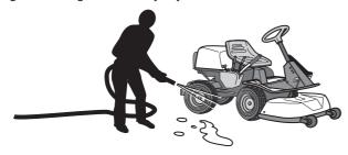
IMPORTANT! Always park the machine on a level surface with the engine OFF before performing any maintenance.
