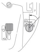
Let the engine run at moderate speed or half throttle for 3-5 minutes before subjecting it to heavy load. When mowing, use 3/4 to full throttle.
