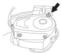
The dipstick should be completely screwed down
