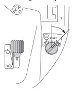
**IMPORTANT INFORMATION** Do not run the starter for more than about 5 seconds at a time. If the engine does not start, wait about 10 seconds before trying again.
