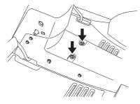
Check the tension of the steering wires by squeezing them together by the arrows as illustrated. It should be possible to push them together so that the distance between them is half as much, without using unnecessary force.
