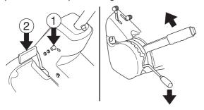
2 Release the clip on the front hood and lift off the fender.
