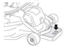
3 Adjust the cutting unit's ground pressure by screwing the adjuster screws, which are located behind the front wheels on both sides, in or out. The ground pressure should be between 12 and 15 kg and the springs evenly tensioned.
