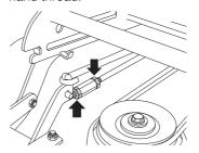
4 Screw out (extend) the stay to raise the rear edge of the cover. Screw in (shorten) the stay to lower the rear edge of the cover.
