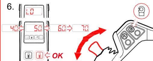
Press the **hook safety lock** button to show the "**LO**" in the display and wait until a value is shown.
