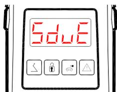
A permanent "**SDUE**" text on the display indicates immediate service. This notification is reset by an authorized HIAB service point in connection with the service.
