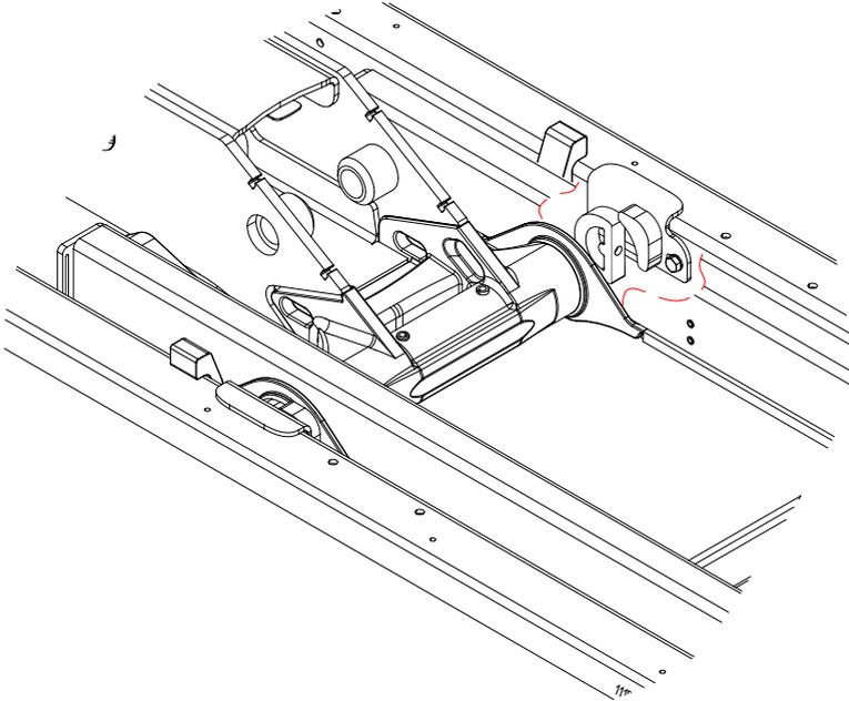
During the lowering of a container, the rear frame is mechanically locked to the auxiliary frame when the middle frame starts to rise. The lock is achieved by the axle tip on the middle frame, which slides under the locking stops in the auxiliary frame.
