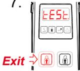
Press the top left button (**locks closed**) to exit from the sub level menu.
