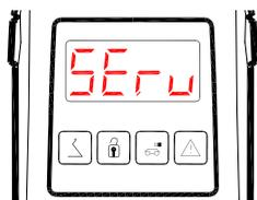
The service interval of the MULTILIFT hooklift is approximately 180 operating hours or 3,600 service cycles, depending on which limit is reached first.
