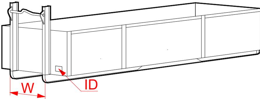
Gripping height (H), tunnel height (T) and width (W) of the container can vary from one container to another. Note that they are country specific dimensions. If there is doubt about the origin of the container, the tunnel height and width must be checked in order to ensure that they are compatible with those of the XR equipment.
