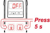
Press both top buttons for 5 seconds to exit the software and return back to normal operation.
