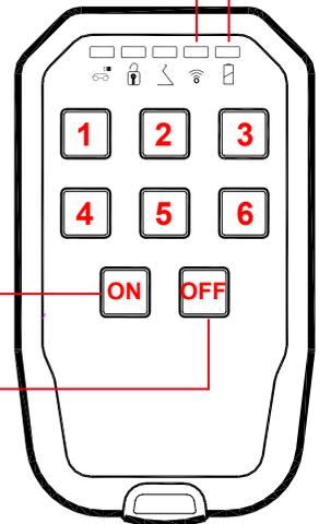
The XR equipment function\*) is activated by simultaneously pressing the **ON** switch and the button for the **function to be activated** (ON+1, ON+2, ON+3, ON+4, ON+5 ja ON+6).
