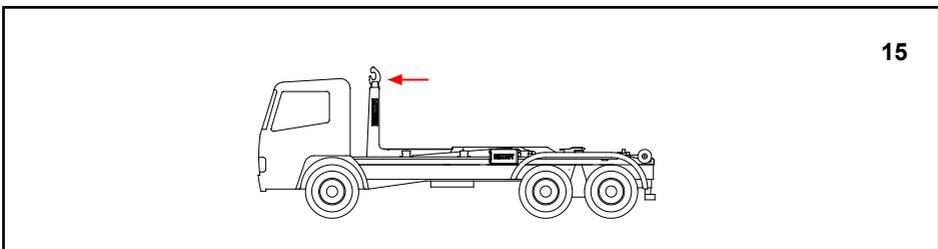
9. **Move the hook arm / middle frame together with the container to rearmost position**
