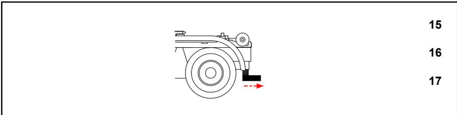
9. **Decrease the speed of tipping movement to prevent an abrupt stop during the last tipping phase.**
