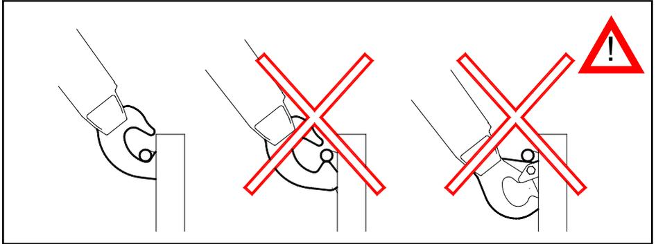
Before picking up the container, the gripping bar of the container must be properly inside the lifting hook. In this way you prevent the container from falling. The situation must be checked by lifting the container approx. 3.9 in (10 cm) and after that checking physically and visually that the container gripping bar is inside the lifting hook.
