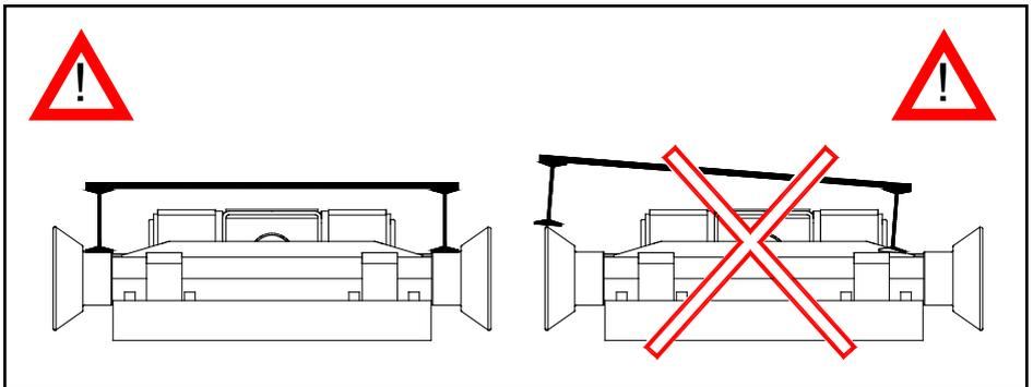
When loading and unloading a container, be sure that it is running in line between the rear rollers.
