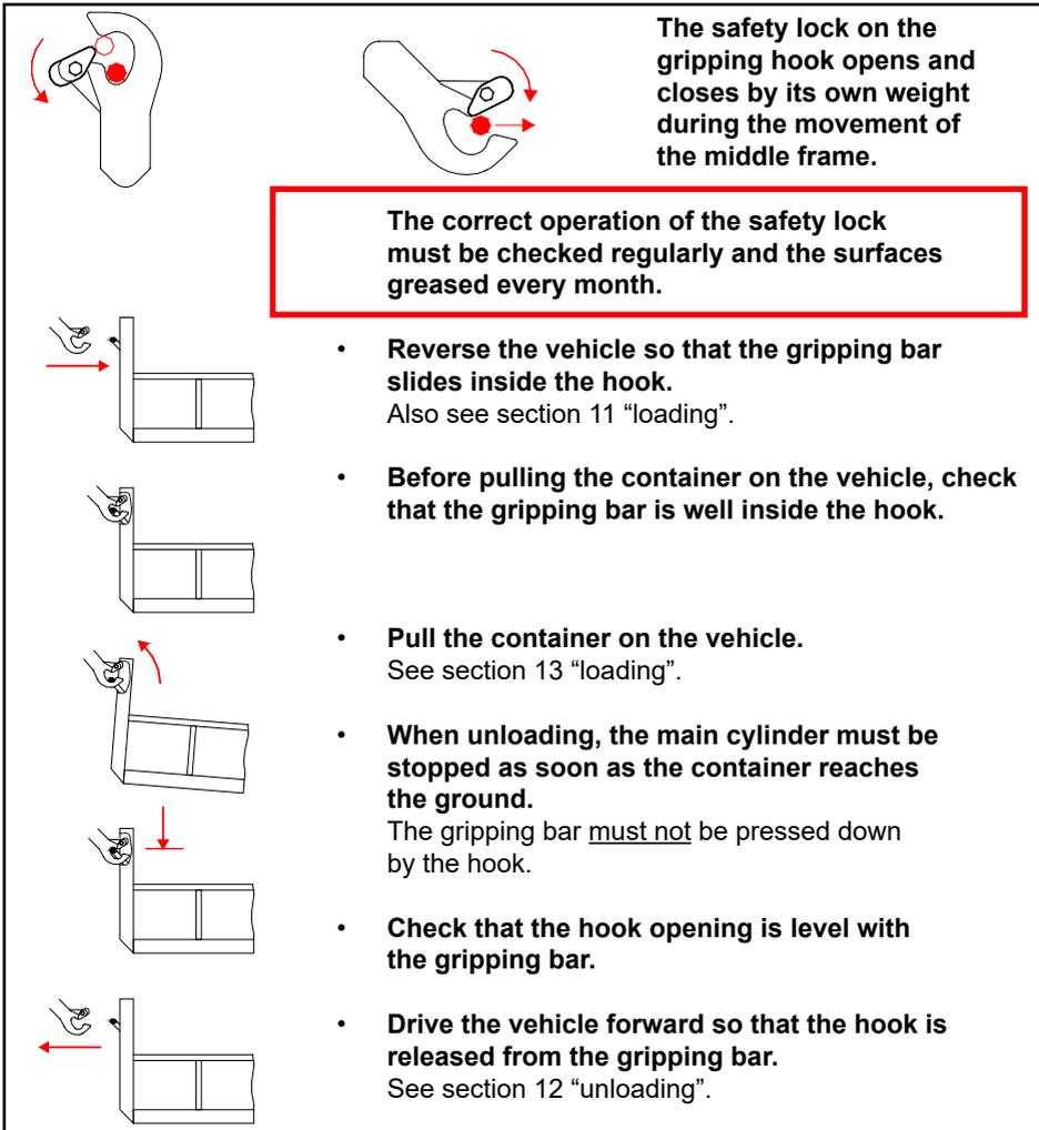
The safety lock on the gripping hook opens and closes by its own weight during the movement of the middle frame.
