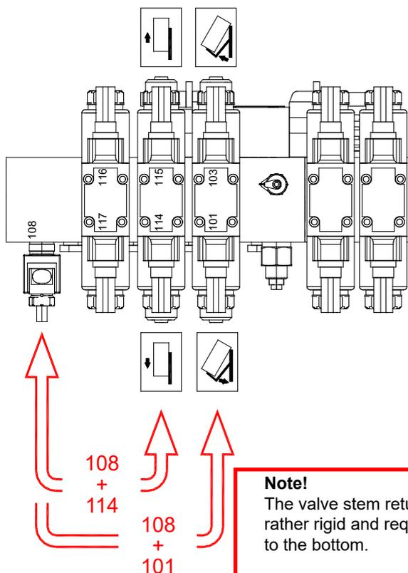
If a failure happens in the electric system of the device, the device may be restored to its normal state, by operating the control valve manually:
