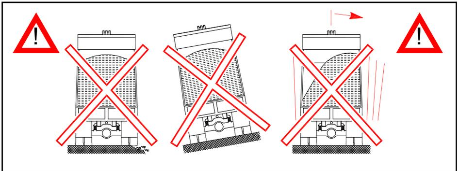
Never load, unload or tip a container when the load is heavier to one side or the ground is sloping.
