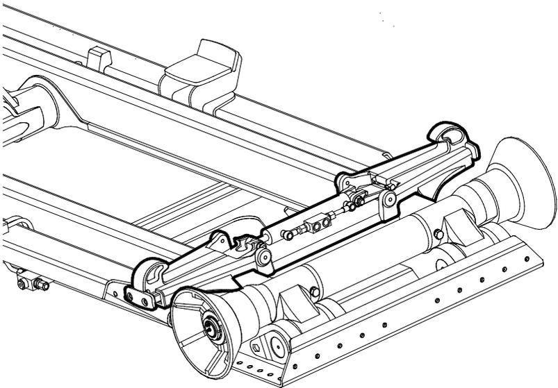
In the outside hydraulic locks, the hooks lock the container in place from the outside flange.
