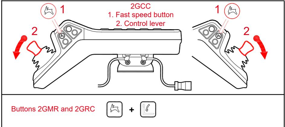
You can use the fast container lowering feature to lower the container faster than normal speed. The speed of the fast lowering is affected by the weight of the empty container and the temperature of the oil; at cold temperatures the speed decreases.
